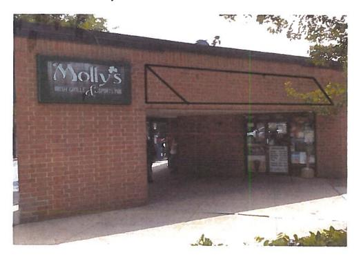
1.Install new awning above opening at 8 4th Street rear. Awning to be the same configuration as 4th Street elevation (There was an awning at this elevation at some point as fasteners are still on building). Awning fabric to match 4th street awning.
